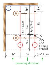
b) Configuration of profiles for alternate mounting of module 600x600mm
