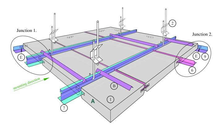
T-profile suspended ceiling frame is manufactured by a number of manufacturers. CEWOOD panel mounting instructions have been elaborated specifically for the frame element system DONN DX-T35. Bearing profiles T 35/38.
