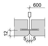
Fig. 4.2. CEWOOD acoustic panel edge profile P5S.
